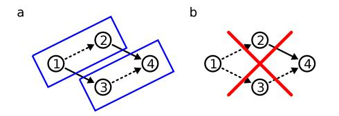
**Figure 3.1:** An example of valid and invalid configurations for dataflows involving StreamEdges. Blue rectangles denote inferred connected components.
